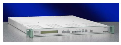
By multiplexing MPEG-2 video content from two ASI inputs to any of four independent RF outputs, the MQAM provides savings both in rack space and cost per video stream over our single-unit QAM. These ASI inputs also allow direct connection to a video server for VOD applications. Under control of the Digital Network Control System (DNCS), the MQAM can be located in either the headend or hub.
